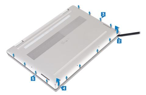
6 Move the base cover from left to right and lift the base cover from the palm-rest and keyboard assembly.
