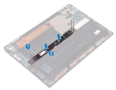
3 Remove the two I/O-board interposers from the system board.
