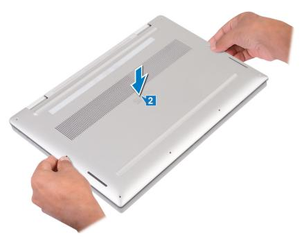
3 Snap the base cover into the tabs on the palm-rest and keyboard assembly.
