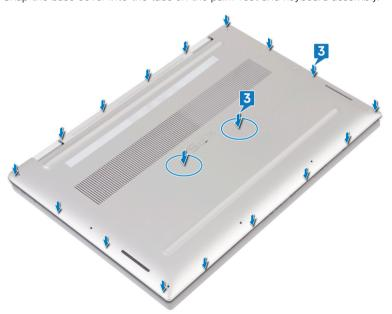
4 Replace the eight screws (M2x3) that secure the base cover to the palm-rest and keyboard assembly.
