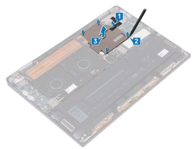
4 In reverse sequential order (as indicated on the heat sink), remove the four screws (M2x3) that secure the heat sink to the system board.
