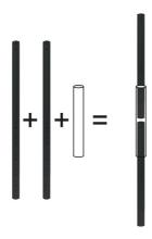
This NewStar flat screen pole connector, model FPMA-CPCONNECTBLACK, allows you to connect multiple poles to stretch the distance from the flat screen to the ceiling using different pole lengths. Ideal with the use of high ceilings.
