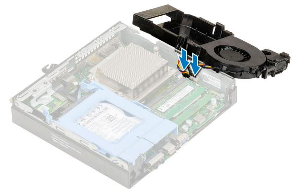
b Place the system fan on the system and slide the system fan until it clicks into place.
