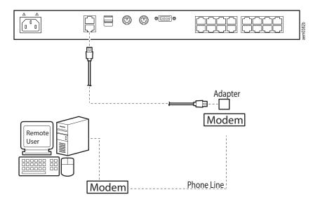
2. From your client computer, use your modem dial-in program to dial into the KVM switch's modem.
