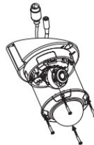
Make sure the rubber stopper is in the side cable channel to seal it.
