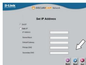
Select **DHCP** if your camera obtains an IP address automatically from a DHCP server such as a router. Select **Static IP** if you want to manually enter the IP settings for the camera.
