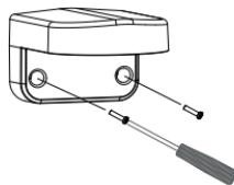
Guide the camera connectors through the back or bottom cable channel on the DCS-37-1. Then screw the mounting plate to the bracket using the set of mounting holes marked **B**.
