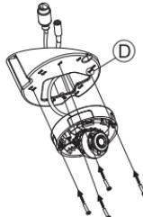
Remove the cover and adjust the angle and rotation of the camera as desired, then put the cover back in place. Screw the camera cover back in place.
