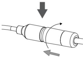
Screw the back part of the waterproof connector clockwise until there is a tight seal around the Ethernet cable.
