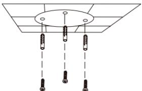
**If you are running the camera cables through the wall,** drill a hole in the center and pull the cables through the hole.
