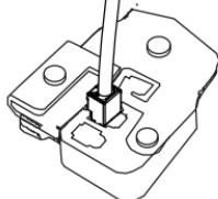
Connect the RJ-45 plug into the Ethernet connector, then screw the waterproof connector to the Ethernet connector by turning it clockwise for about a half-turn.
