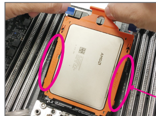
CPU Rail Frame Rails
