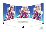
IPS displays use advanced technology that gives you extra-wide viewing angles of 178/178 degrees, making it possible to view the display from almost any angle — even in 90-degree Pivot mode! Unlike standard TN panels, IPS displays gives you remarkably crisp images with vivid colours, making it ideal not only for
