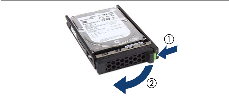
Figure 24: Opening the 2.5-inch HDD/SSD module locking lever
