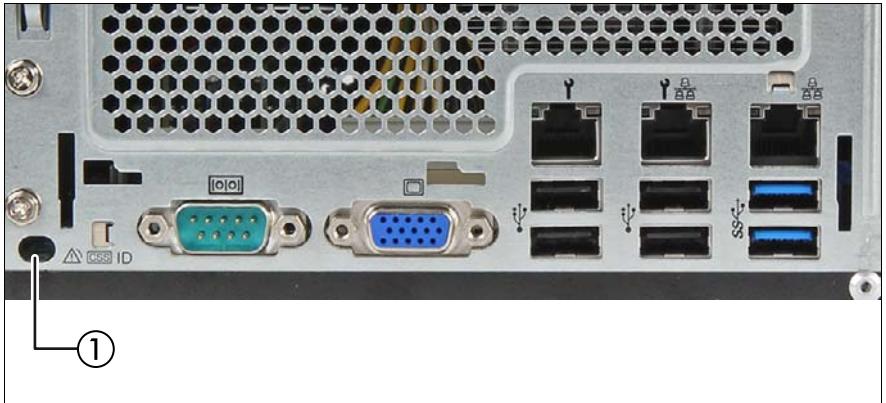
Figure 9: ID, CSS and Global Error indicators
