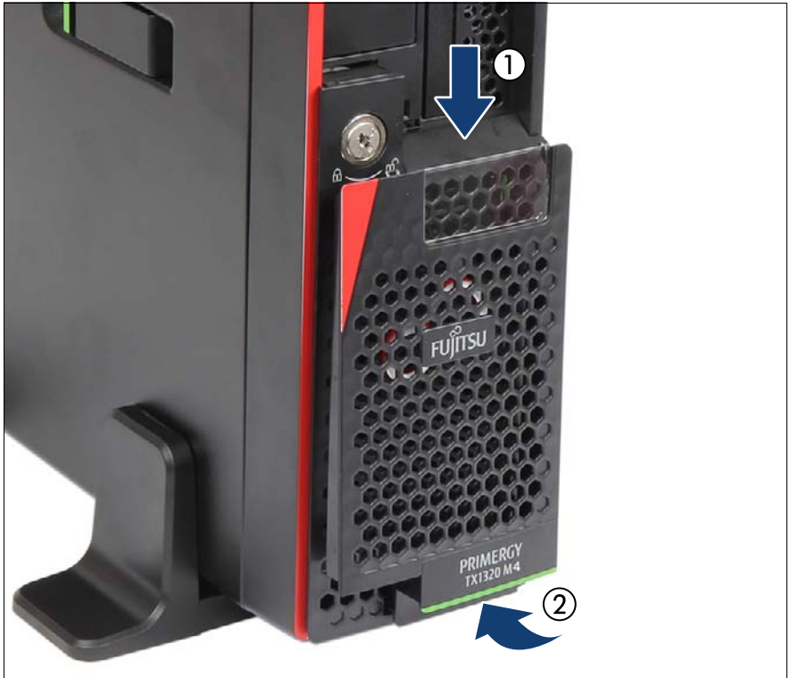
Figure 21: Placing the drive cover in front of the HDD cover
