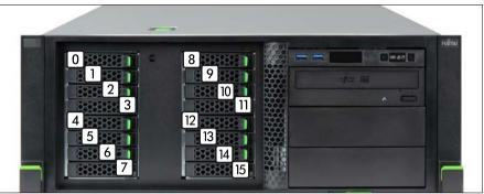
Figure 119: Configuration with up to 16 2.5-inch HDDs/SSDs
