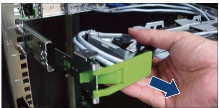
Figure 71: Removing the CMA stopper
