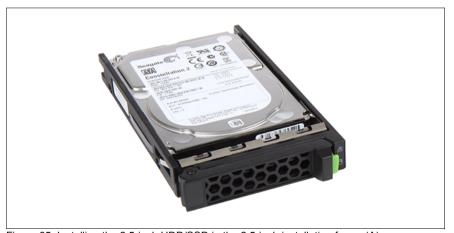
Figure 85: Installing the 2.5-inch HDD/SSD in the 2.5-inch installation frame (A)
