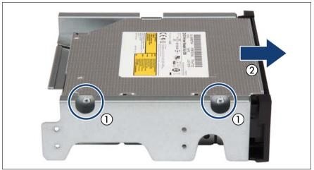
Figure 265: Removing the ultraslim ODD from the ultraslim ODD adapter
