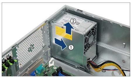
Figure 58: Taking out the standard PSU
