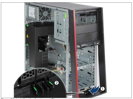
Figure 28: Installing the front cover (B)
