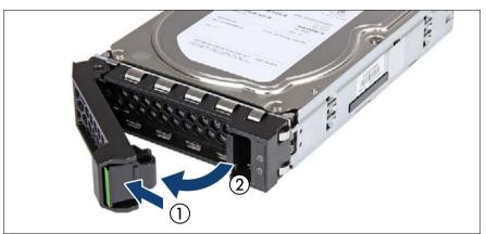
Figure 99: Opening the 3.5-inch HDD module locking lever
