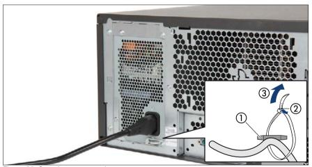
Figure 35: Securing power cord
