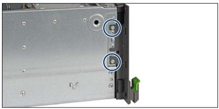
Figure 9: Removing the rack front cover (A)
