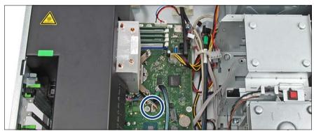
Figure 37: Disconnecting the fan cable
