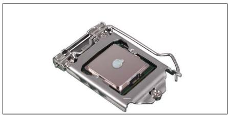
Figure 226: Applying thermal paste
