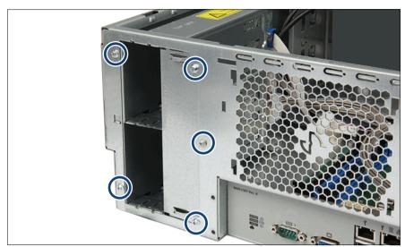
Figure 82: Securing the PSU cage
