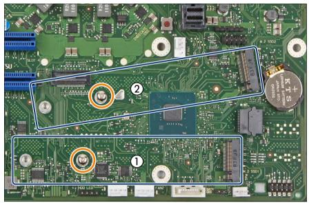
Figure 285: Slots for M.2 SSDs
