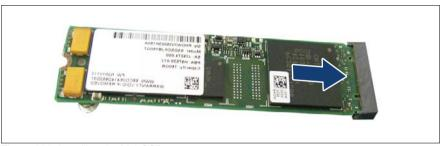
Figure 286: Installing the M.2 SSD
