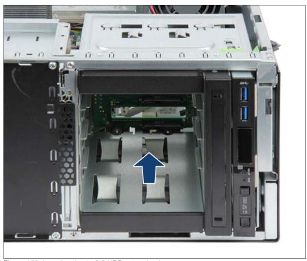
Figure 156: Inserting the 4x 3.5 HDD extension box
