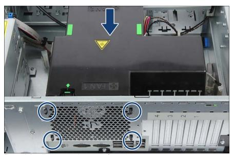
Figure 43: Installing the redundant system fan module
