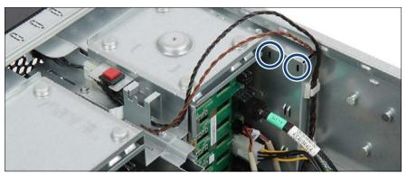
Figure 167: Installing the SAS expander holder (A)
