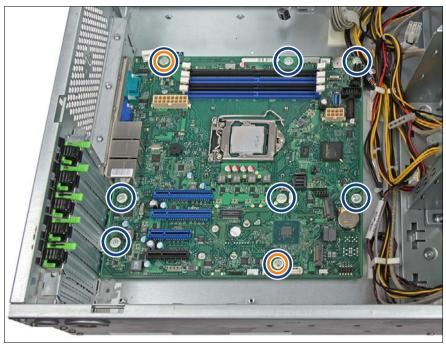
Figure 296: Screws system board
