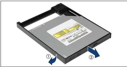
Figure 253: Removing the slimline ODD from its installation frame
