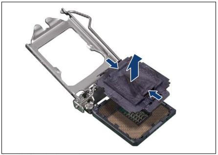
Figure 234: Removing the protective cover
