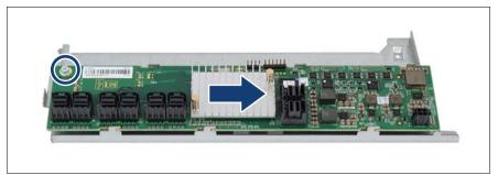
Figure 170: Removing the SAS expander board
