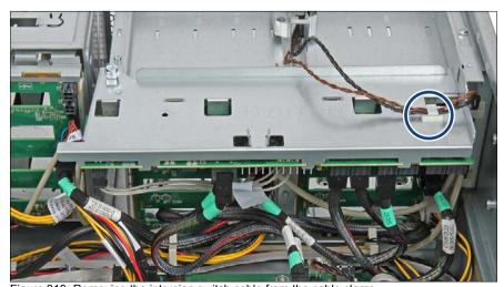
Figure 313: Removing the intrusion switch cable from the cable clamp
