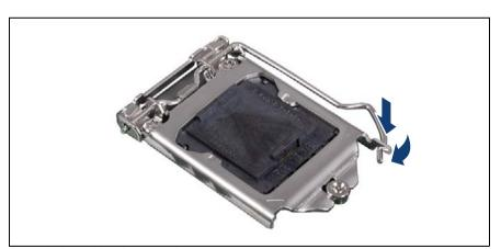
Figure 231: Latching the socket lever
