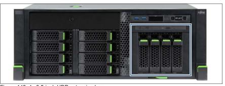
Figure 143: 4x 3.5-inch HDD extension box
