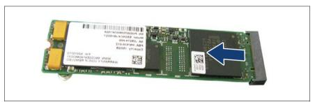
Figure 289: Removing the M.2 SSD (B)
