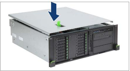
Figure 23: Installing the top cover (rack server) (A)
