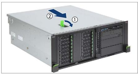
Figure 24: Installing the top cover (rack server) (B)
