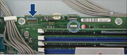
Figure 292: Installing the Dual microSD 64GB Enterprise
