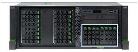
Figure 142: 8x 2.5-inch HDD/SSD extension box
