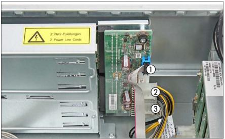
Figure 78: Connecting the power distribution board
