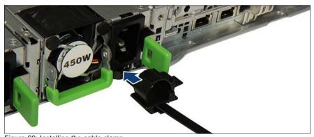
Figure 69: Installing the cable clamp
