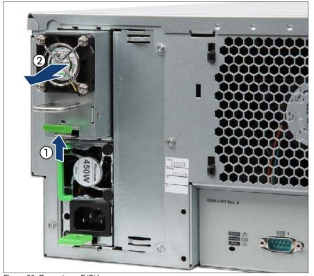
Figure 80: Removing a FJBU
