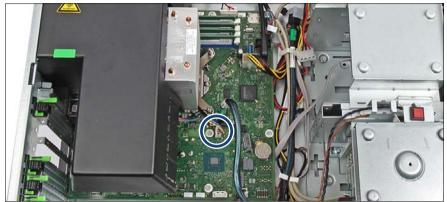
Figure 42: Connecting the system fan cable
