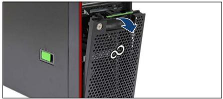
Figure 17: Removing the HDD bay cover
