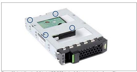
Figure 89: Installing the 2.5-inch HDD/SSD in the 3.5-inch installation frame (B)
