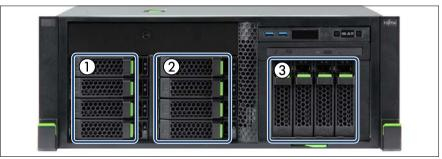
Figure 92: 3.5-inch HDD SAS backplanes - rack model
