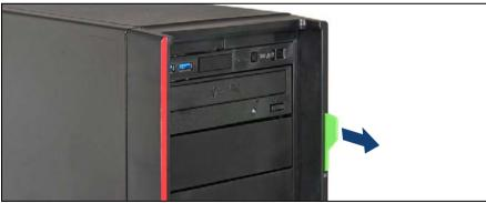
Figure 18: Removing the ID card (floorstand model)
