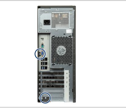
Figure 300: Removing the right side cover (A)
