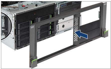
Figure 20: Installing the rack front cover
