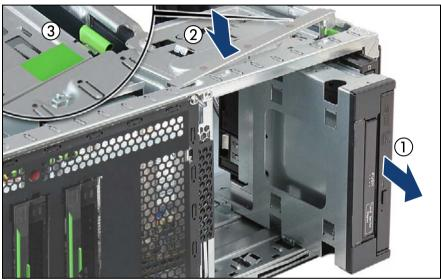
Figure 251: Removing the Multibay box
