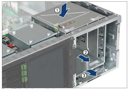
Figure 307: Mounting the accessible drive cage
