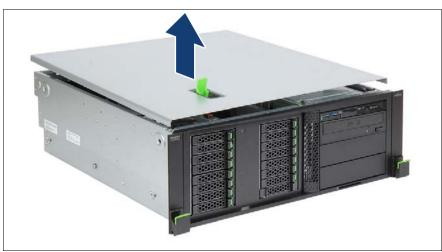
Figure 7: Removing the top cover (rack server)
