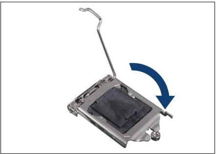
Figure 229: Closing the load plate (A)
