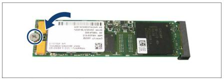
Figure 287: Fastening the M.2 SSD
