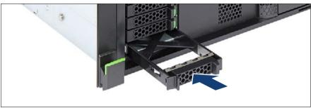
Figure 125: Installing a 2.5-inch HDD/SSD dummy module
