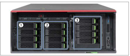
Figure 93: 3.5-inch HDD SAS backplanes - floorstand model
