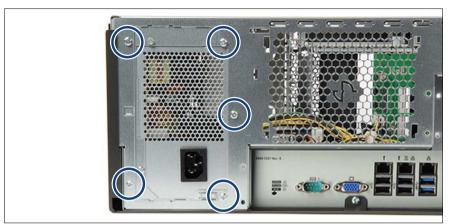
Figure 57: Removing the screws
