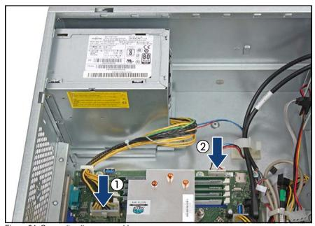
Figure 64: Connecting the power cables
