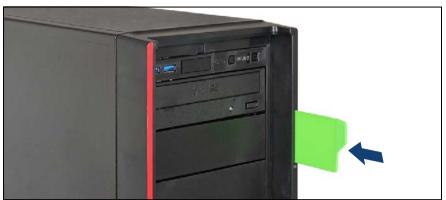
Figure 29: Installing the ID card (floorstand model)
