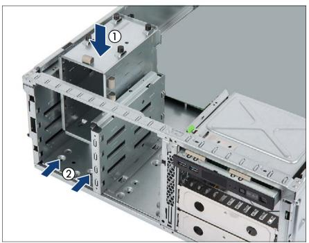
Figure 134: Installing the 2.5-inch HDD/SSD cage
