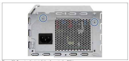
Figure 62: Securing the installation frame to the PSU
