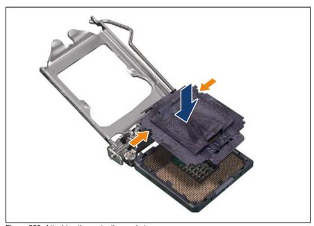
Figure 228: Attaching the protective socket cover
