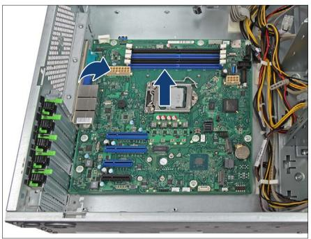
Figure 297: Removing the system board
