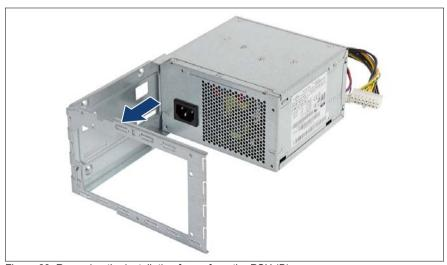
Figure 60: Removing the installation frame from the PSU (B)
