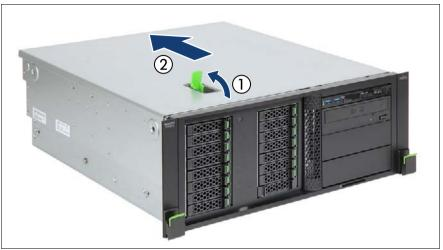
Figure 6: Removing the top cover (rack server)
