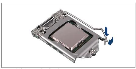
Figure 224: Closing the socket release lever
