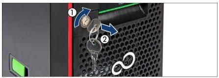
Figure 13: Unlocking the server
