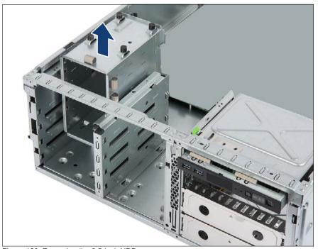
Figure 129: Removing the 2.5-inch HDD cage
