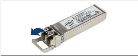
Figure 182: Unlatching the locking bail
