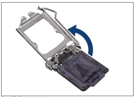
Figure 233: Opening the load plate
