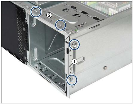
Figure 304: Detaching the accessible drive cage (B)
