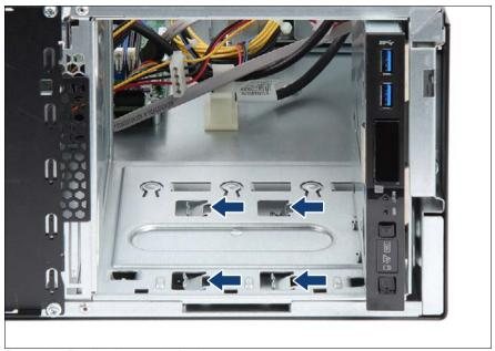
Figure 155: Bending in mounting brackets
