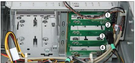
Figure 111: Connecting cables to the SAS backplane (example 4. 3.5-inch HDDs)
