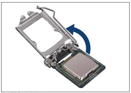
Figure 219: Opening the load plate
