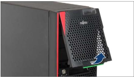
Figure 15: Removing the accessible drive bay cover
