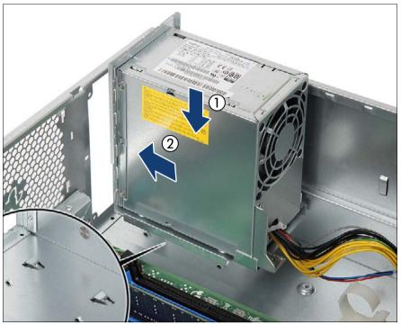
Figure 63: Installing the standard PSU
