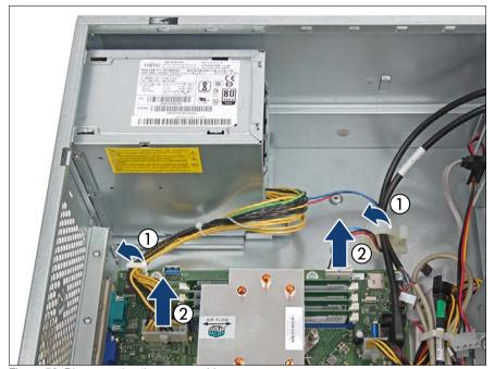
Figure 56: Disconnecting the power cables
