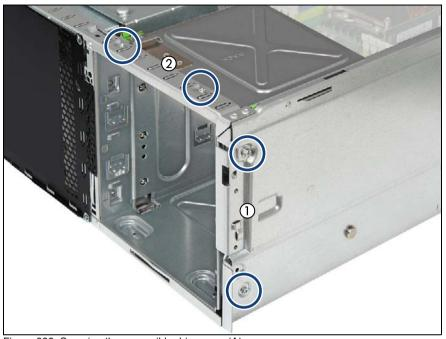
Figure 308: Securing the accessible drive cage (A)
