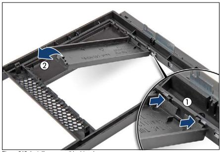
Figure 312: Installing accessible drive dummy covers
