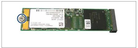
Figure 288: Removing the M.2 SSD (A)
