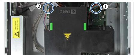
Figure 39: Disconnecting the fan cables
