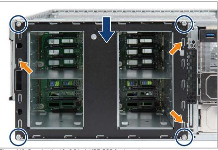
Figure 140: Securing the 16x 2.5-inch HDD/SSD front panel
