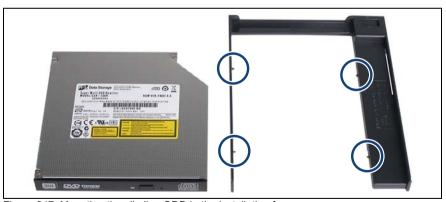
Figure 247: Mounting the slimline ODD in the installation frame
