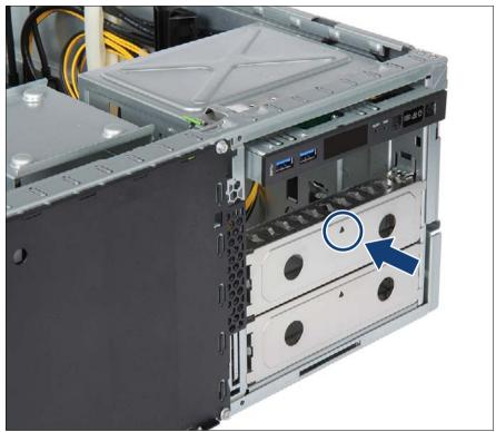
Figure 50: Installing an accessible drive filler cover
