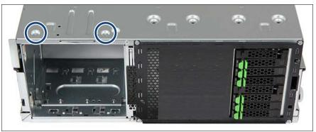
Figure 303: Detaching the accessible drive cage (A)
