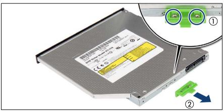
Figure 261: Removing the locking latch from the ultraslim ODD
