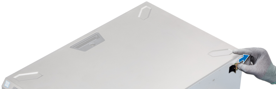
Figure 121. Attaching the mylar cover
