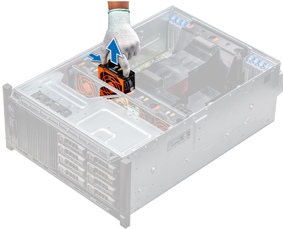
Figure 21. Removing a middle cooling fan
