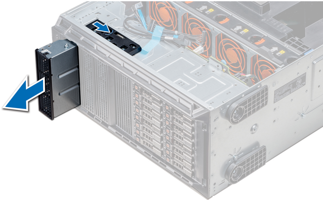
Figure 59. Removing the optical drive or tape drive
