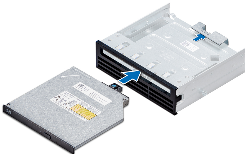
Figure 64. Installing the slim optical drive blank
