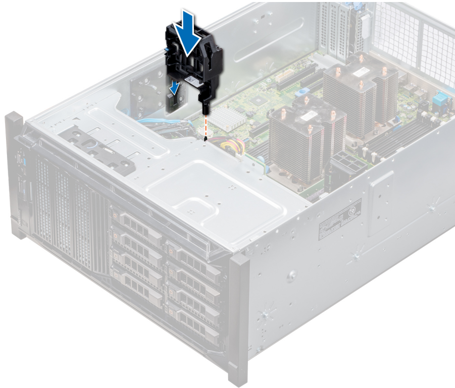
Figure 80. Installing the optional GPU card holder
