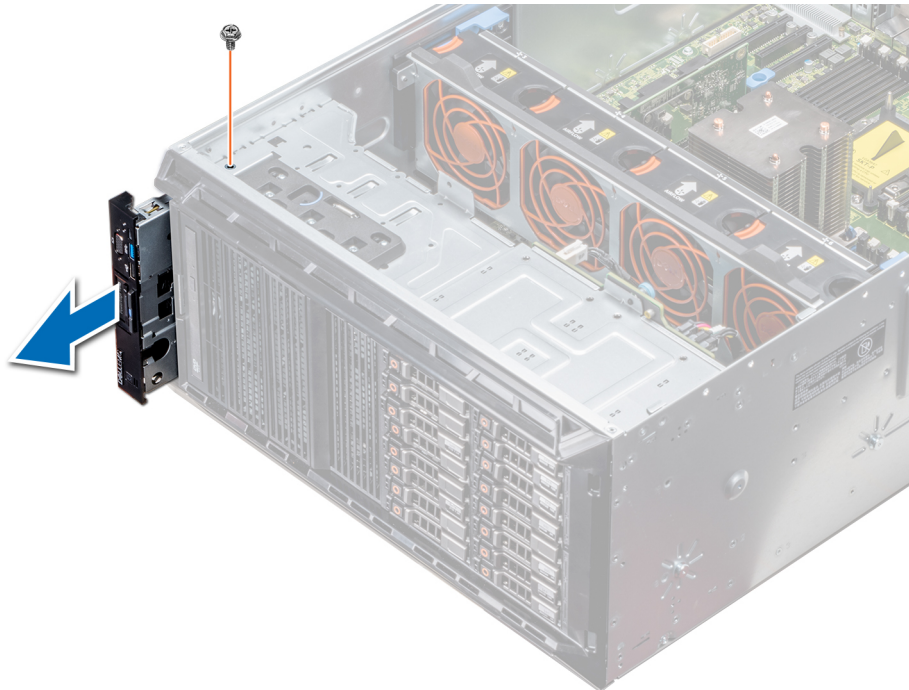
Figure 106. Removing the control panel assembly
