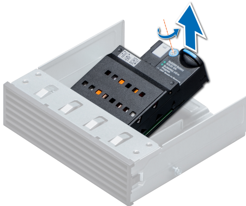
Figure 65. Removing the NVDIMM-N battery
