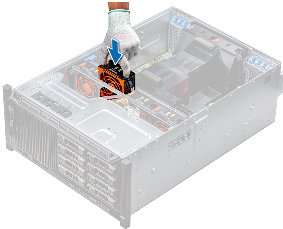
Figure 22. Installing a middle cooling fan
