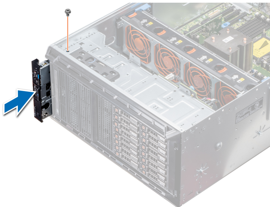
Figure 109. Installing the control panel assembly
