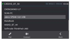
6. Once paired successfully, touch the Connect softkey to connect the remote device; "Connected" is displayed alongside the device:
