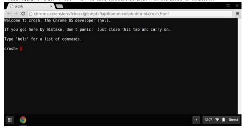
Type in the CROSH command for diagnostics. Type 'help' for a list of available commands. Type help\_advanced to display a complete list of commands for debugging purposes
