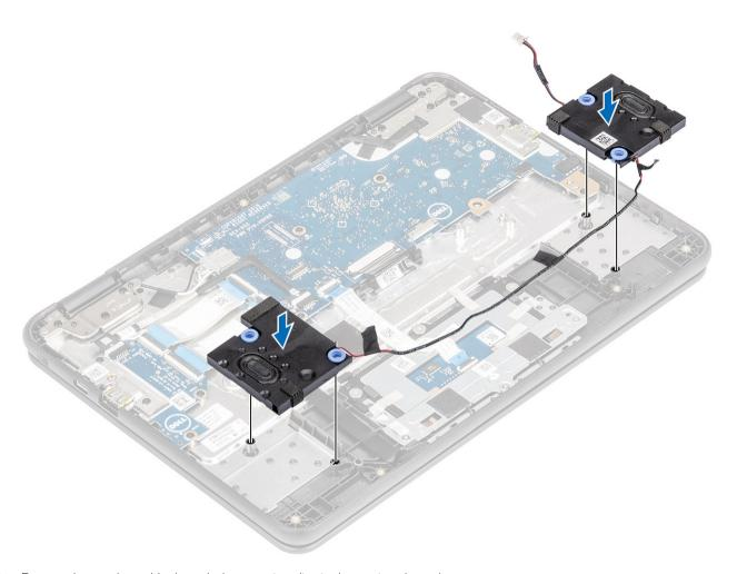
Reroute the speaker cable through the retention clips in the routing channel. 2
