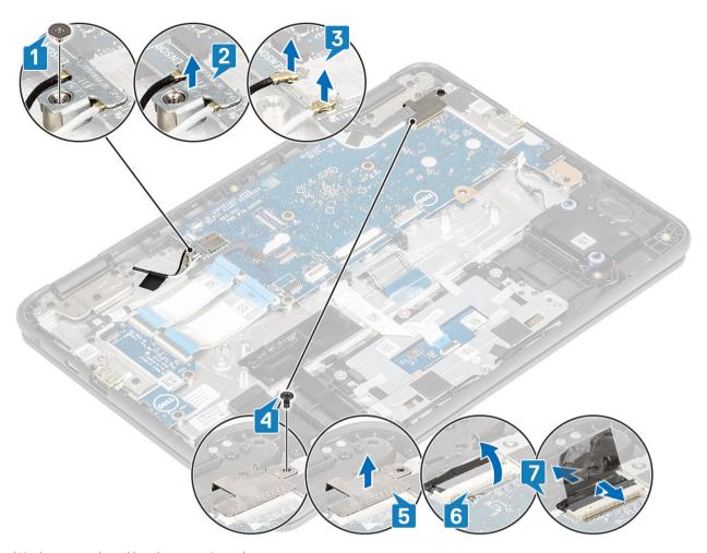
Lift the system board bracket away from the computer.
