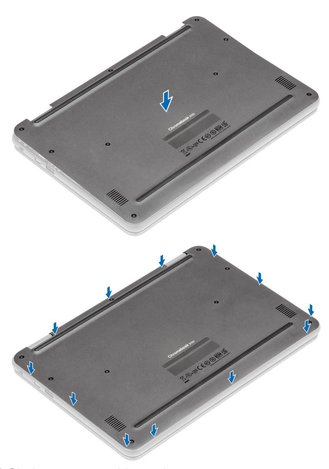
2 Tighten the nine captive screws to secure the base cover to the computer.
