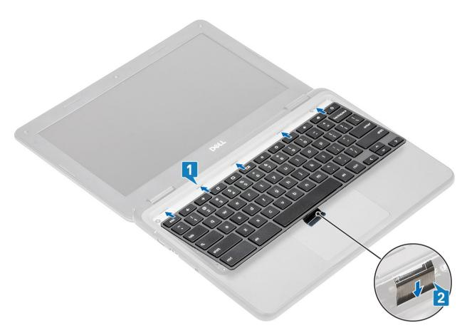
2 Press the keyboard until it clicks into place and then close the LCD fully before turning the system over [1, 2]
