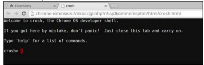
5 Type battery\_test 1 into CROSH, and then press Enter.
