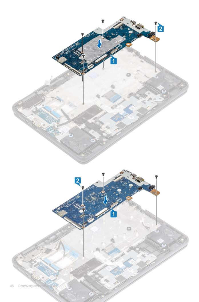
3 Place the IO board bracket in its place on the system board.
