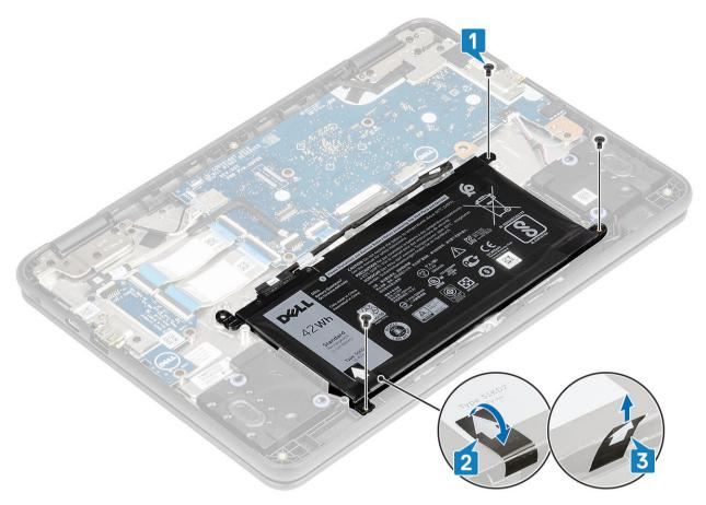
Pry the battery from the bottom edge [1] and remove the battery from the computer [2].
