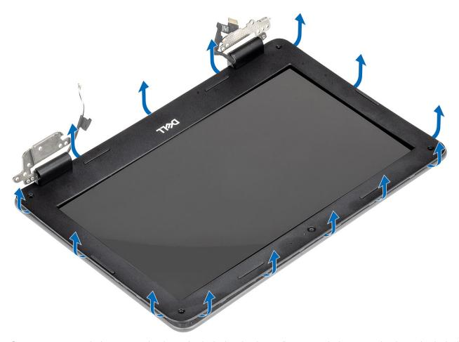
4 Continue to pry open the bottom outside edge of the display bezel and carefully pry open the bottom inside edge of the display bezel.
