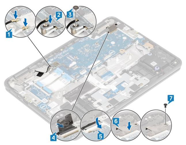
7 Connect the Type-C power cable and the speaker cable to the connectors on the system board [1, 2].
