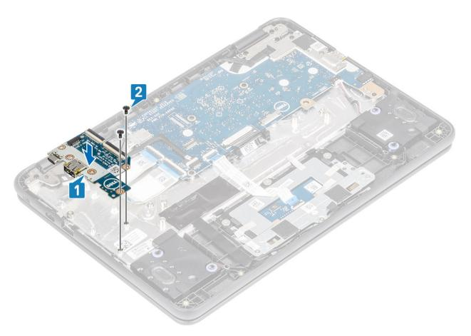
Place the IO board bracket to its slot and replace the two (M2.0x4.0) screws that secure the bracket to the IO board [1, 2].
