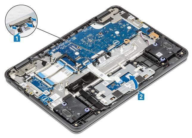
3 Use a plastic scribe to release the keyboard from the two release holes in the system [2].
