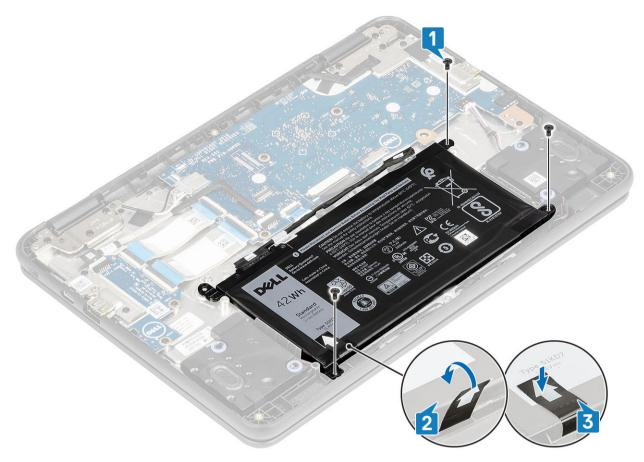
5 Reroute the battery cable and connect the cable to the connector on the system board [1, 2].
