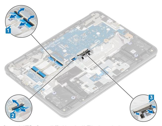
Disconnect the USB Type-C power cable [1] and the speaker cable [2] from the system board. 2
