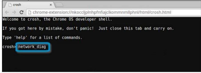
Wait while CROSH performs a set of network diagnostic tests. A diagnostic screen displays the results of the network adapter health test.
