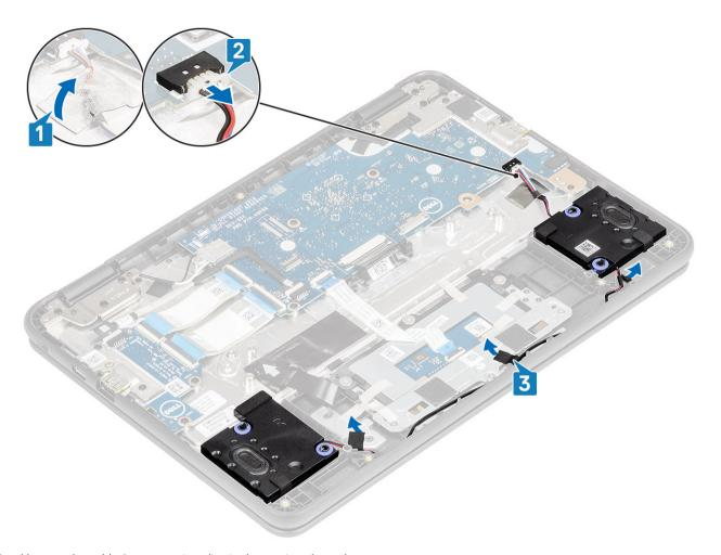
4 Unroute the cable from retention clips in the routing channel.
