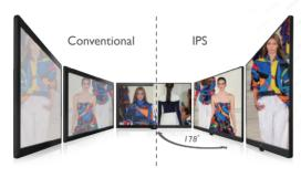
IIPS (In-Plane Switching) Technology provides accurate color and image reproduction from any angle. An expansive 178° viewing angle is ideal for work and for on-screen reviews with multiple people in the room.
