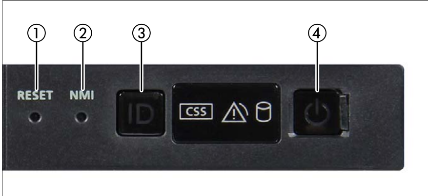
Figure 6: Controls on the front panel module
