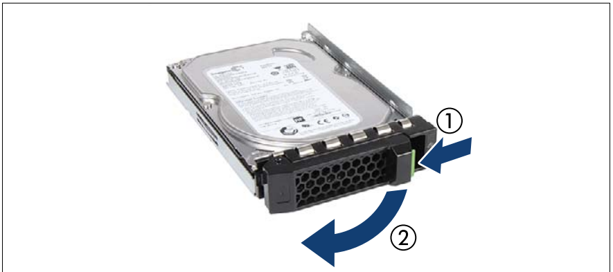
Figure 25: Opening the 3.5-inch HDD module locking lever
