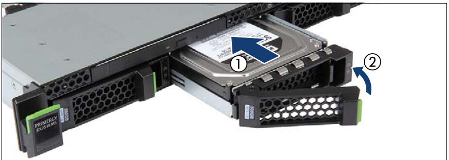
Figure 26: Installing the 3.5-inch HDD module
