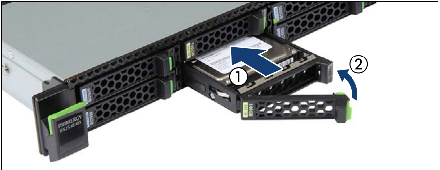
Figure 29: Installing the 2.5-inch HDD/SSD module
