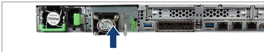
Figure 34: Installing an FJBU
