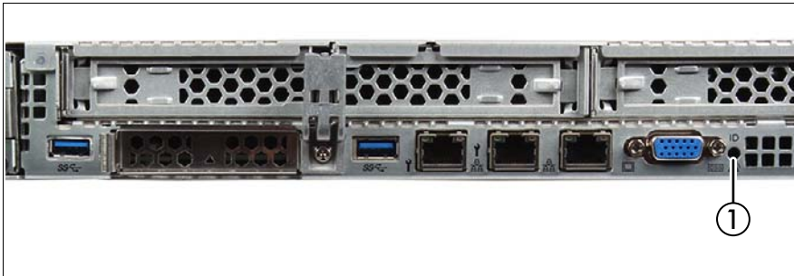
Figure 12: Indicators on the I/O panel: ID, CSS and Global Error indicators
