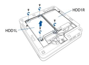
6. (optional) To upgrade your HDD/SDD, first remove the four (4) screws on the bracket, then remove the bracket.
