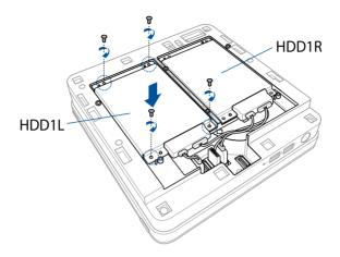
**NOTE:** Ensure to organize the cables to prevent any damage to your VivoMini and to ensure the top cover can be replaced successfully.
