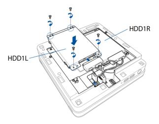
**NOTE:** Ensure to organize the cables to prevent any damage to your VivoMini and to ensure the top cover can be replaced successfully.
