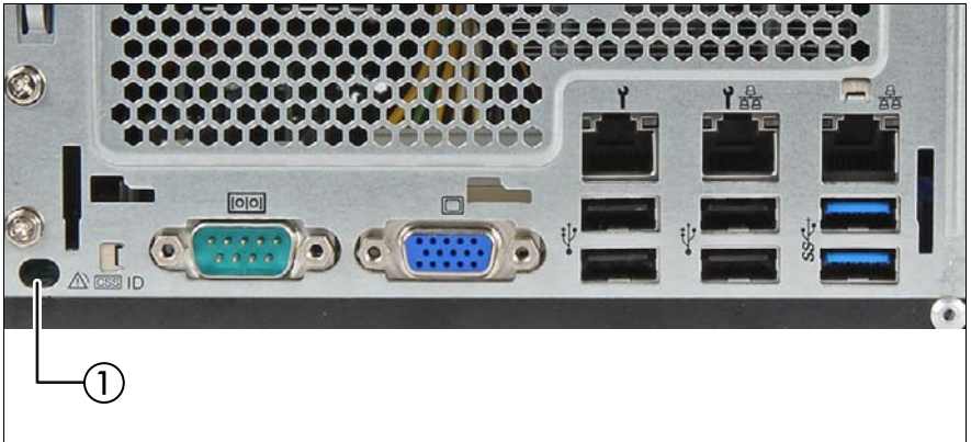
Figure 9: ID, CSS and Global Error indicators
