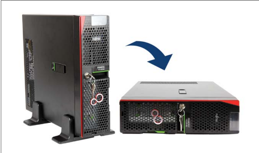
Figure 17: Positioning the server horizontally
