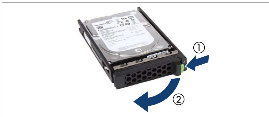
Figure 24: Opening the 2.5-inch HDD/SSD module locking lever
