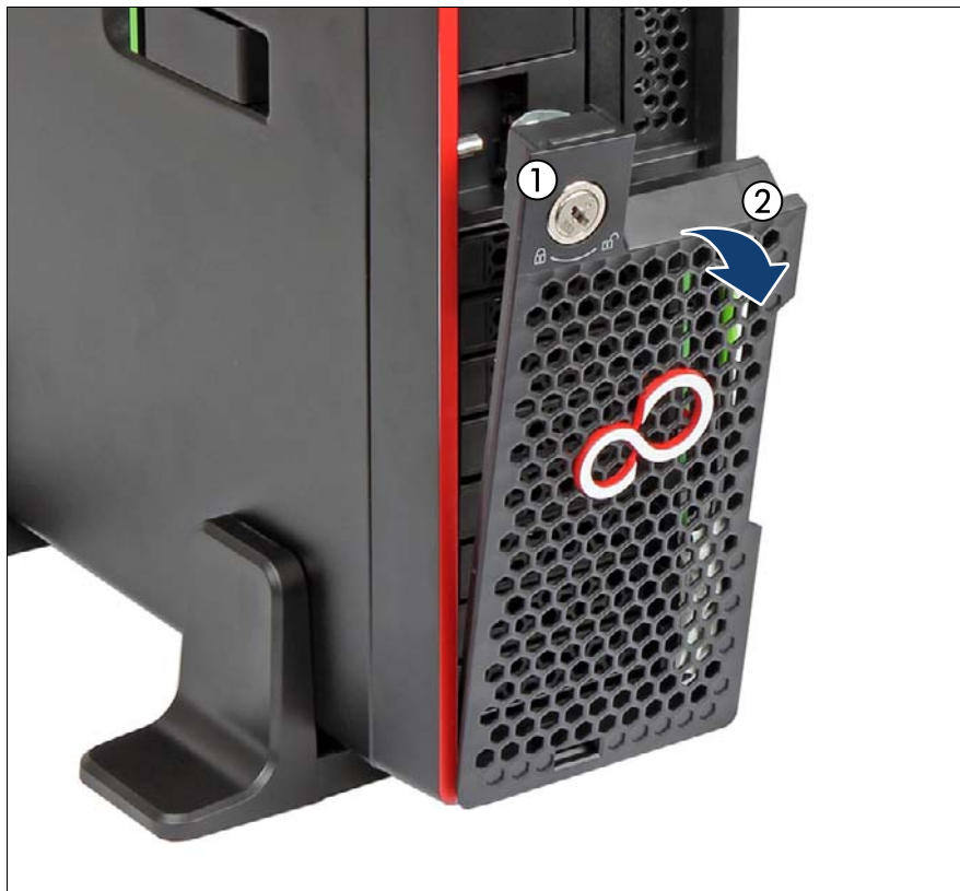
Figure 22: Removing the HDD cover
