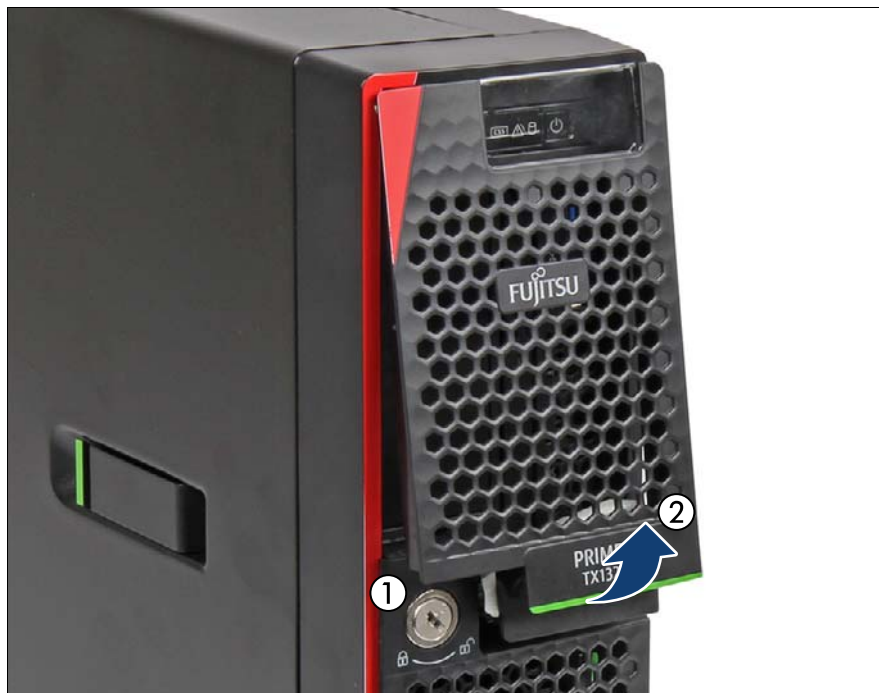
Figure 20: Removing the drive cover
