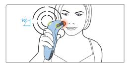
Flickering green light and humming sound: the laser is interrupted. Make sure the application tip has full skin contact, is at the right angle and is being moved at the right speed.
