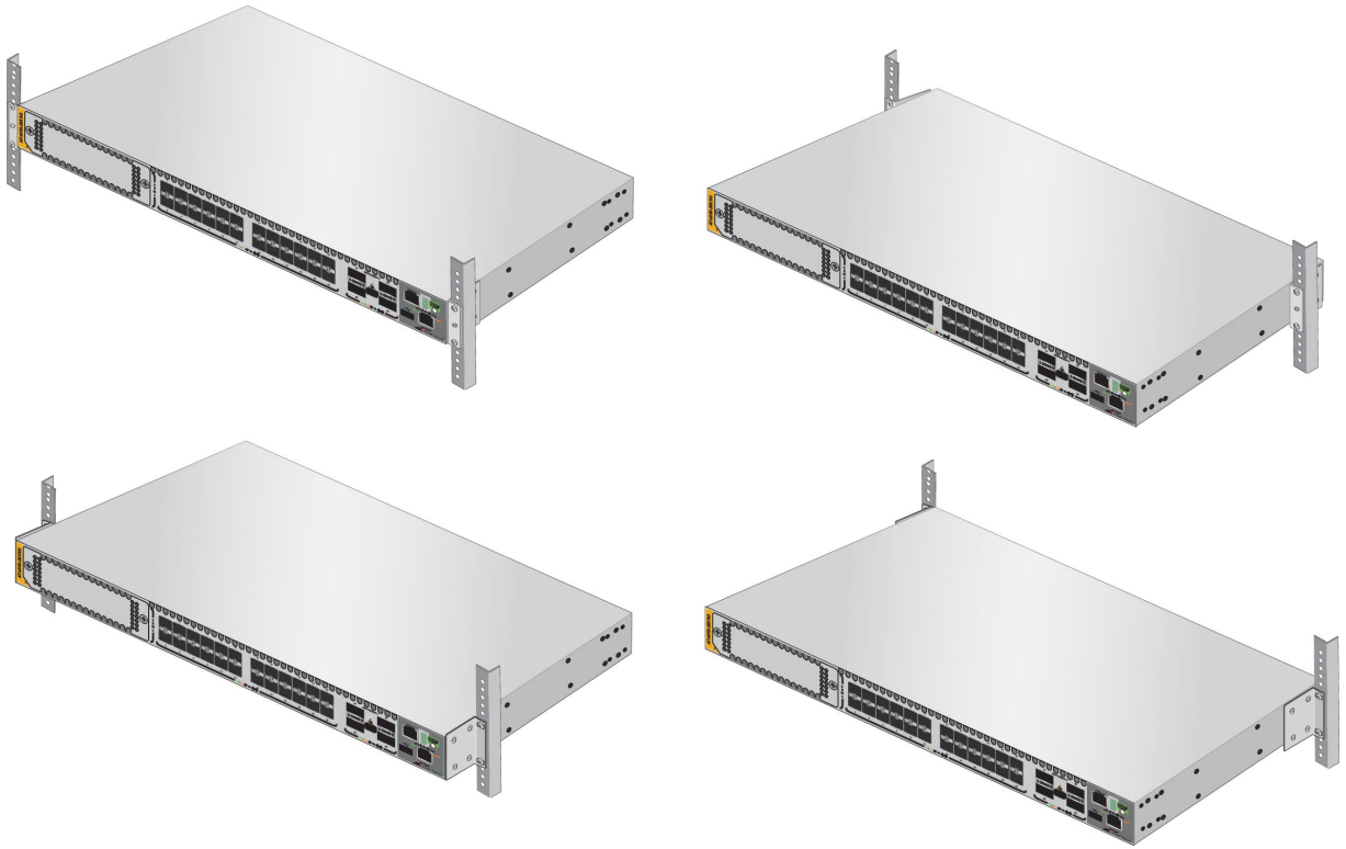
Figure 65. Switch Orientations in an Equipment Rack
