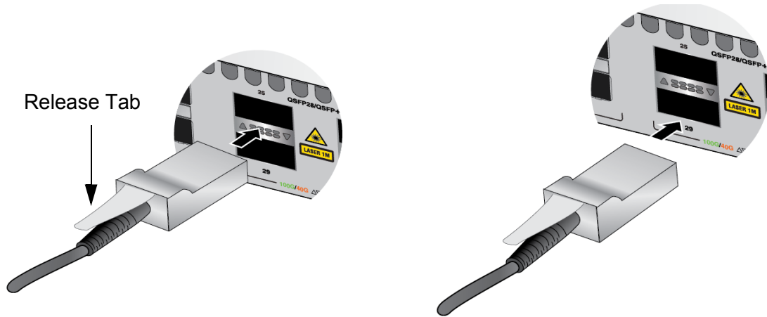
Figure 121. Attaching QSFP+ Cables
