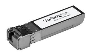
The SFP-10G-BX-D-20-ST is a Cisco SFP-10G-BX-D-20 compatible downstream fiber SFP+ transceiver which pairs with StarTech.com's SFP-10G-BX-U-20-ST. They are designed, programmed and tested to work with 10GBase-BX compatible Cisco switches and routers. The SFP+ transceiver module supports a maximum distance of up to 20 km (12.4 mi) and delivers dependable 10 GbE connectivity over fiber cabling.
