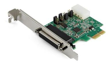
This PCI Express RS232 serial adapter card lets you add four RS232 (DB9) serial ports to your computer through a PCI Express (PCIe) slot, as if they were native serial ports. The 4 port PCIe serial card enables you to interact with serial devices, such as card readers, printers, PIN pads, and modems, at speeds of up to 921.6Kbps.
