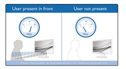
PowerSensor is a built-in 'people sensor' that transmits and receives harmless infrared signals to determine if a user is present and automatically reduces monitor brightness when the user steps away from the desk, cutting energy costs by up to 65 percent and prolonging monitor life
