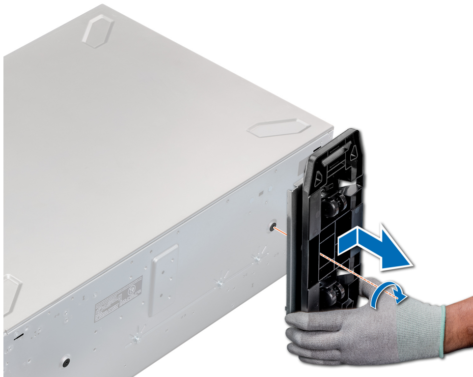
Figure 30. Installation des roulettes
