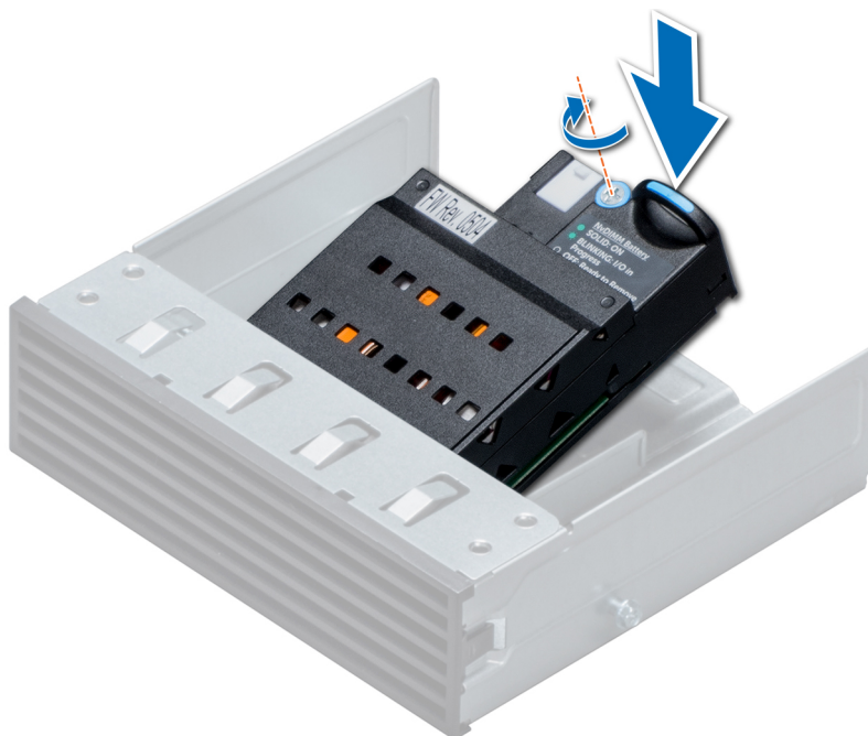
Figure 66. Installation de la pile NVDIMM-N
