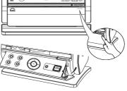
Insert the USB device's USB plug into the socket on the set 's foldable control panel
