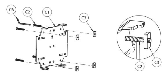
ii. Slide *item C1* down the front slots of *item A1* to the correct height and tighten *items C2*. **Note:** Space the 2 mounting plates (*item C1*) 600mm apart on each column.
