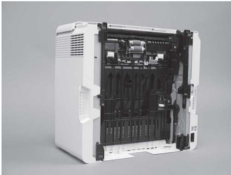
Figure 6-14 Place the printer bottom-side face forward
