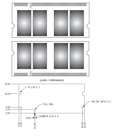
Figure 1: KVR533D2S4/512 200-Pin SODIMM
