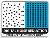
During weak signal transmission, random noise will appear on the image. When viewed, the image contains dark and white dots. Noise reduction significantly reduces the appearance of these dots, hence creating a pleasant viewing experience
