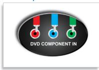
Component Video is the highest quality interconnection standard for analog video. It is sharper than S-video and composite video
