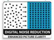
During weak signal transmission , random noise will appear on the image. When viewed, the image contains dark and white dots. Noise reduction significantly reduces the appearance of these dots , hence creating a pleasant viewing experience
