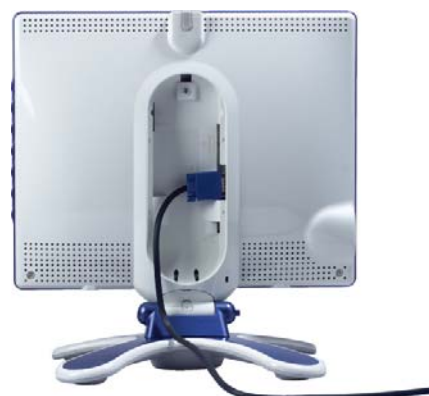
VGA D-Sub Cable (blue plug)
