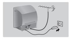
• Insert the aerial plug into the **T** socket at the rear of the set.
