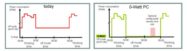
The graphics explain the principle theory of operation. The 0-Watt PC can automatically switch the PC to zero watt without using a mechanical power switch or switchable power strip. The power supply of the PC disengages its internal circuits from the power plug upon the entrance of the 0-Watt mode
