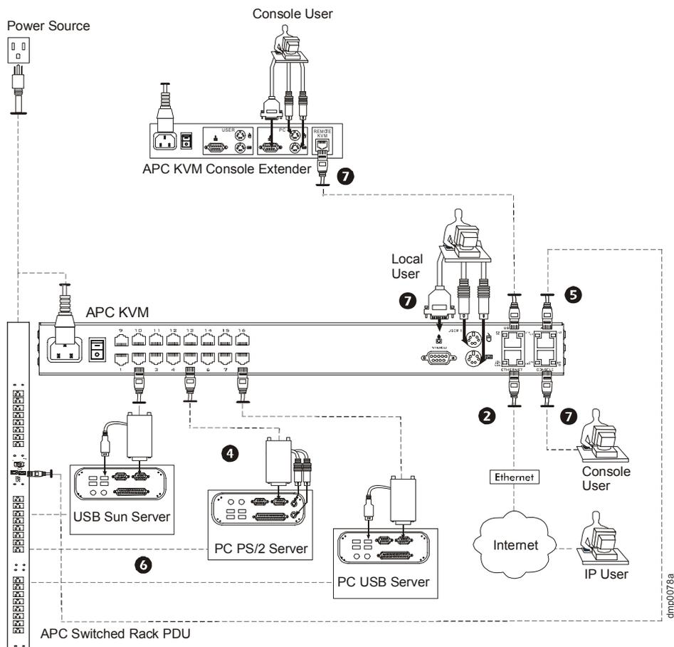
The following table lists the basic installation instructions in the order they should be performed. For detailed information about a procedure, see the page number listed for that step.
