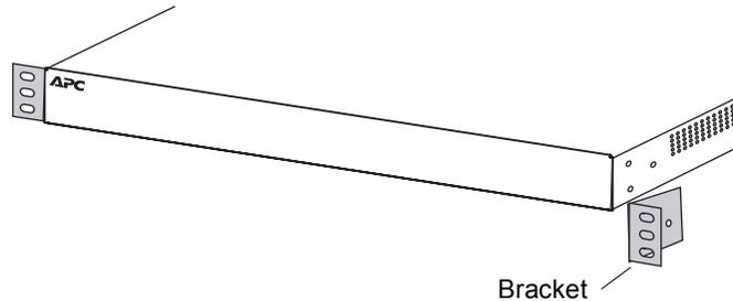
3. Use the mounting hardware recommended for your rack to mount the IP KVM.
