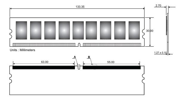
Figure 1: KVR800D2E5/1G 240-Pin DIMM
