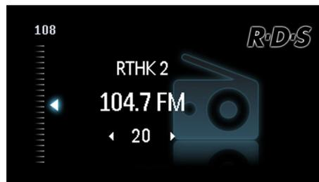
RDS (Radio Data System) is a communications protocol standard that allows digital information to be transmitted over FM radio broadcasts. RDS-enabled FM radio receivers can display this useful information that includes station identity,
