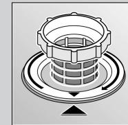
Screw in filter system NOTE MARK!
