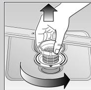
Rotate filter cylinder, remove filter system ...
