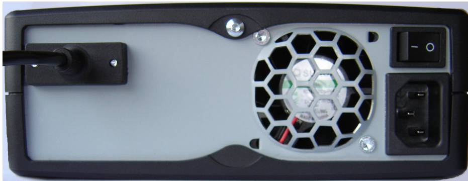
Figure 13. New DAT enclosure with quieter fan
