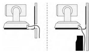
6. Attach the camera to the mount using the 1/4"-20 x .375 mounting screw supplied with the camera.
