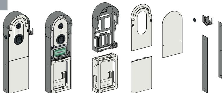
The necessary components for assembling the EVlink Pro AC Metal are the following:
