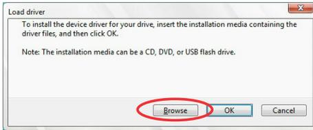
5. Locate the driver in the corresponding folder of the Support DVD or the USB flash drive with RAID driver, then click **OK** to continue.
