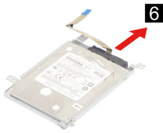
Figure 45. Remove the HDD cable
