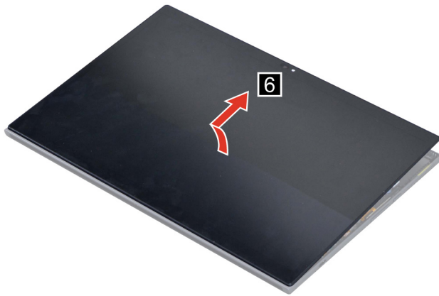
Figure 5. Lift the LCD module.
