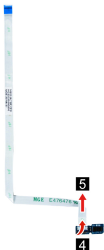
Figure 31. Separate the ToF cable from the ToF board.
