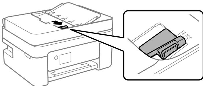
4. Place the originals face-up and short edge first in the ADF, and then slide the ADF edge guide to the edge of the originals.
