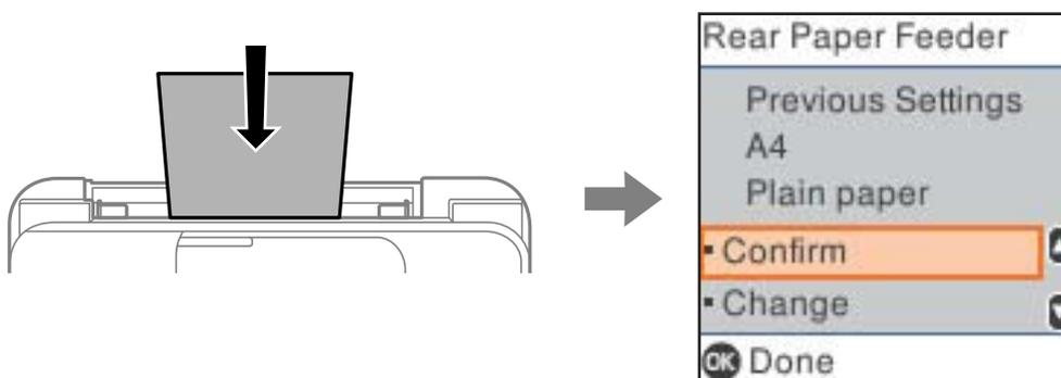
If displayed paper size and type differ from the loaded paper, select **Change** to make changes. Select the paper size and paper type, check the settings, and then press the OK button. If the settings match the loaded paper, select **Confirm**.
