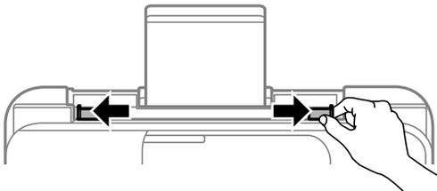
3. Load paper at the center of the paper support with the printable side facing up.
