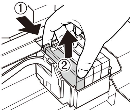
6. Insert the new ink cartridge, and then press it down firmly.
