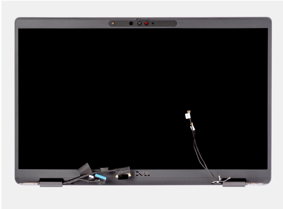
Figure 3. Display assembly with WWAN-antenna cables
