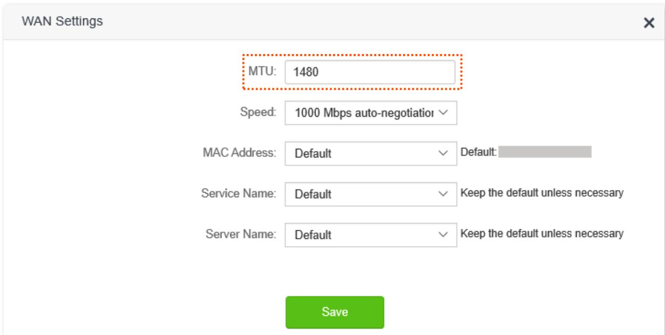
The screenshot shows the WAN Settings configuration page. The MTU field is highlighted with a red dashed box and contains the value 1480. Other fields include Speed (1000 Mbps auto-negotiation), MAC Address (Default), Service Name (Default), and Server Name (Default). A green Save button is at the bottom.
