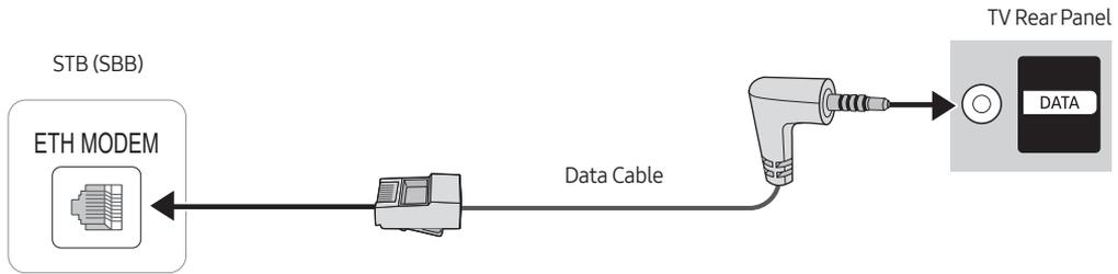
Connect the **DATA** port of the TV to the **ETH MODEM** port of the STB (SBB) with the Data cable.
