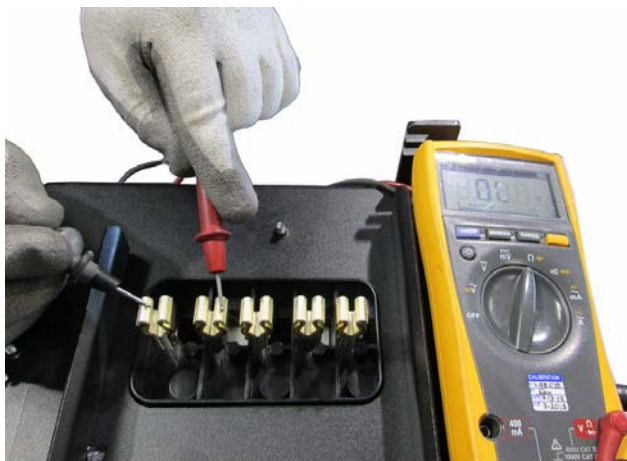
Figure 5: Testing for Plug-In Unit Isolation Prior to Installation
