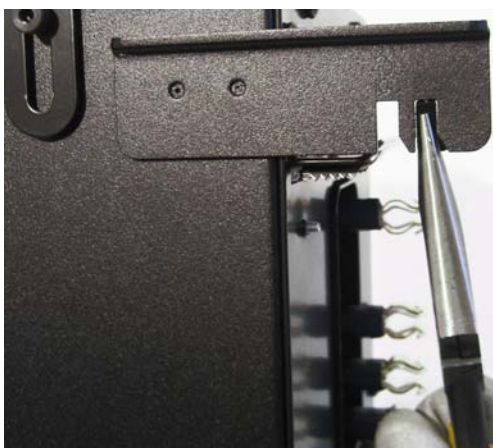
Figure 10: Removing 225 A Knockout
