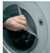
3 | Once the clamp is removed, detach the flap from the gasket, to allow access to the inside of the product
