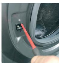
4 | By using Torx wrench, remove the fixing screws of the door lock
