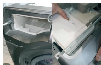
6 | Disassemble the dispenser and bezel
