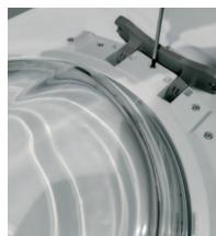
4 | Remove all the screws of the porthole
