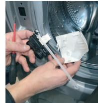
9 | Replace the door lock by paying attention to mechanical linkage of emergency opening and electrical connections
