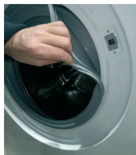
**3** Once the clamp is removed, detach the flap from the gasket, to allow access to the inside of the product
