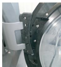
4 | Pull the porthole from the top and remove it
