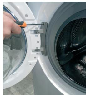
**2** By using the 25 Torx wrench, remove the screws that fix the hinge to the cabinet
