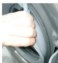
7 | Once the strap is removed, detach the flap from the gasket, to allow access to the inside of the product
