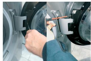
2 | Remove the cover after removed its screw
