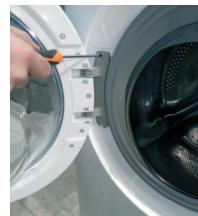
2 | By using the 25 pipe wrench, remove the screws that fix the hinge to the cabinet
