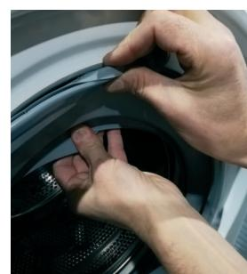
**8** Tighten the clamp flush on the tube by using the tooling
