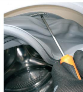
**4** By using flat screwdriver, remove the clamp on the tube
