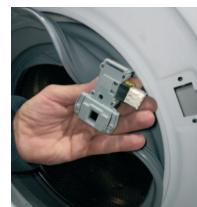
6 | Disconnect the wiring, in case of "faston", pay attention to do not invert the wiring
