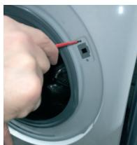
4 | By using Torx wrench, remove the fixing screws of the door lock, and press its buckle.
