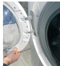
3 | Pull the porthole from the top and remove it
