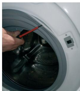
**2** Use the flat screwdriver for leverage, and remove the external clamp
