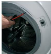
2 | Use the flat screwdriver for leverage, and remove the external clamp
