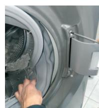
8 | Remove the external screws from the hinge
