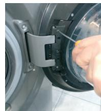
3 | Remove the screws of the plastic hinge
