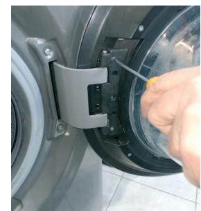
**3** Remove the screws of the plastic hinge
