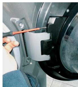
**2** Remove the cover after removed its screw
