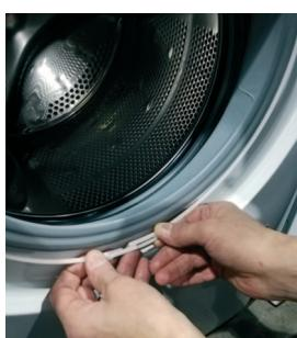
**9** Fit the gasket on the cabinet. Fix the external clamp and tighten it (if needed with tong)
