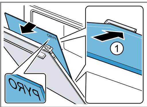
5. Push the inner pane in at the top ①. Push the sliding caps **a** downwards in the direction of the arrow.
