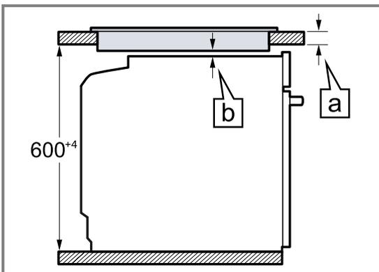
The minimum worktop thickness  $\boxed{a}$  is based on the required minimum clearance  $\boxed{a}$ .
