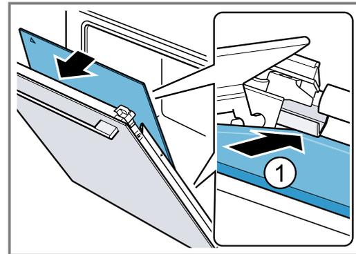
2. **Note:** The intermediate pane is automatically positioned by the rotational movement of the spacer. Slide the second intermediate pane into the central retainer ① and fit it at the top.
