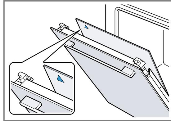
1. Slide the first intermediate pane into the lowest retainer ① and fit it at the top.
