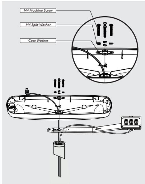
**7** Attach the Case and Self-Service Mount to the Mounting arm with the 20mm M4 Machine Screws (supplied with Self Service Mount).
