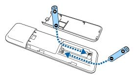
**Warning:** Make sure the batteries are inserted in the correct positions. If the batteries are not inserted correctly, they could explode or leak, causing a fire, injury, or damage to the product.
