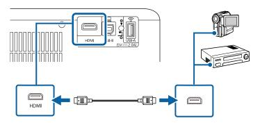
**Note:** When an audio/video source that meets the HDMI CEC standard is connected to the projector's HDMI port, you can use the projector's remote control to control certain features of the linked device by accessing the **Settings > Operation** menu and enabling the **HDMI Link** setting.
