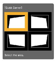
6. Use the arrow buttons on the remote control to select the corner of the image you want to adjust. Then press **Enter**.
