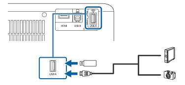
3. If you connected a USB cable, connect the other end to the USB device as necessary.
