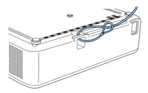
2. Attach the other end of the safety wire to a structure that is strong enough to bear the projector's weight. If the wire is too long, loop the wire around so that there is as little slack as possible.
