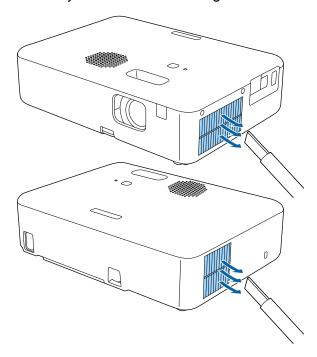
**Caution:** Do not use canned air. The gases may leave a flammable residue or push dust and debris into the projector's optics or other sensitive areas.
