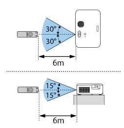
**Note:** Avoid using the remote control in conditions with bright fluorescent lights or in direct sunlight, or the projector may not respond to commands. If you will not use the remote control for a long time, remove the batteries.
